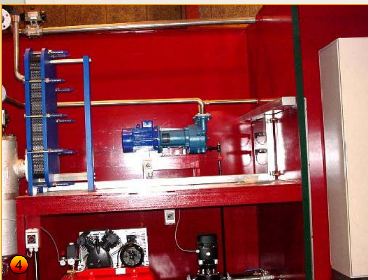
3-5: Compact equipment platform for the complete pump and valve unit, incl. of the electrical cabinet
